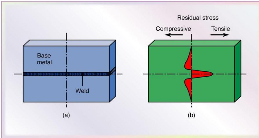
Residual stresses developed in a straight butt joint. Note that the residual stresses in (b) must be internally balanced.
