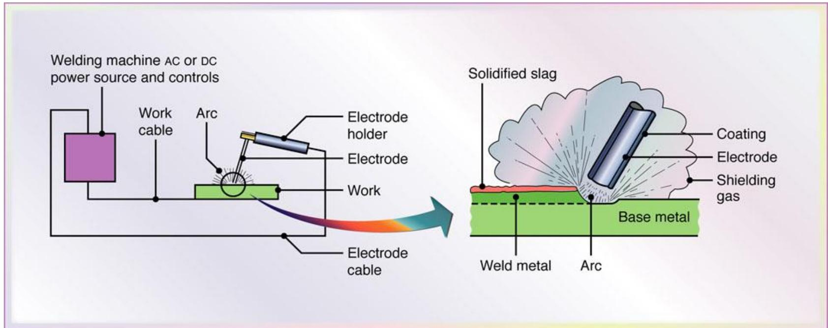
Schematic illustration of the shielded metal-arc welding process. About 50% of all large-scale industrial welding operations use this process.
