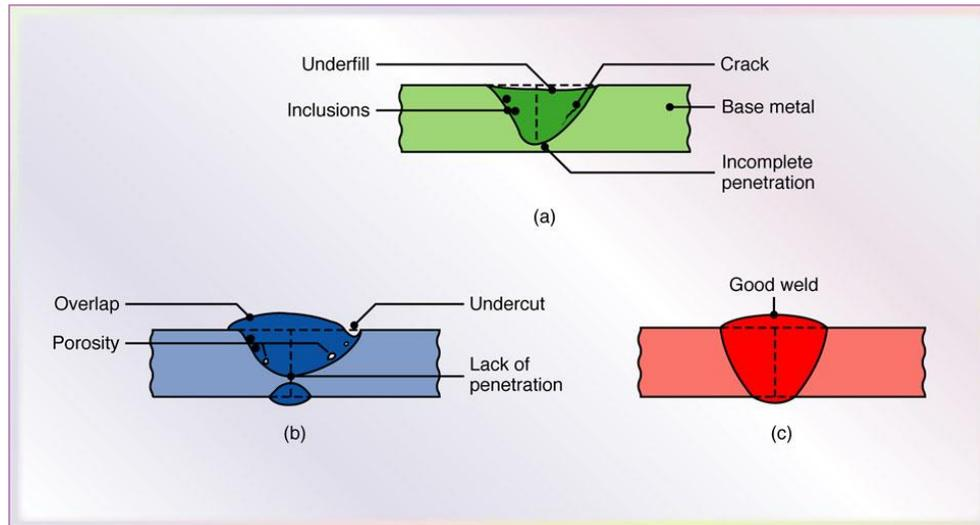
Examples of various defects in fusion welds.
