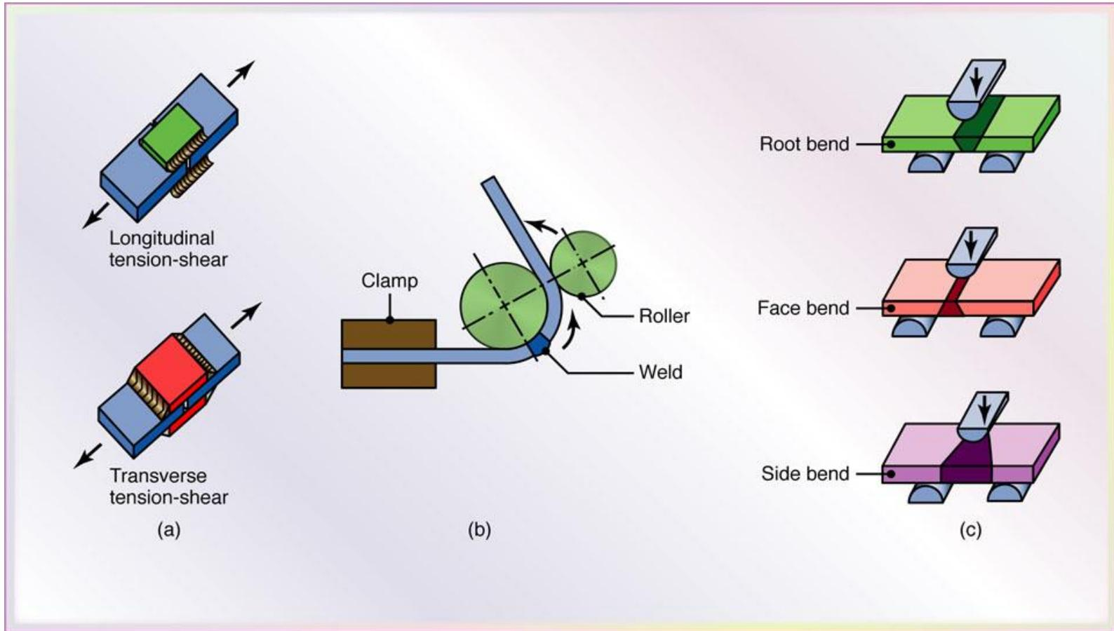
(a) Specimen for longitudinal tension-shear testing; specimen for transfer tension-shear testing; (b) wraparound bend test method; (c) three-point bending of welded specimens.
