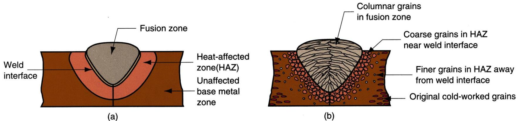
Cross section of a typical fusion welded joint:
