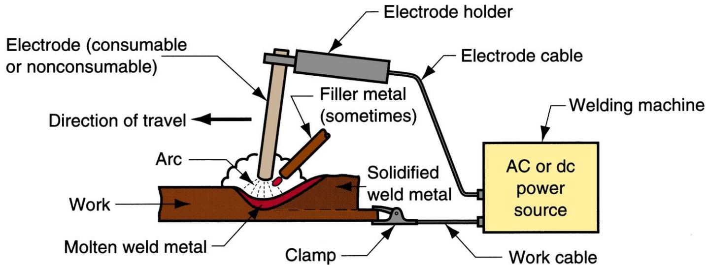
The basic configuration and electrical circuit of an arc welding process
