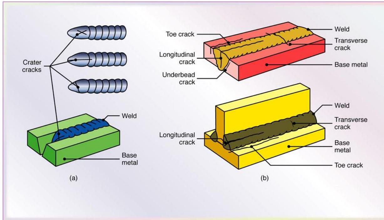
Types of cracks developed in welded joints. The cracks are caused by thermal stresses, similar to the development of hot tears in castings.
