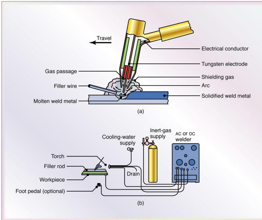
(a) The gas tungsten-arc welding process, formerly known as TIG (for tungsten inert gas) welding. (b) Equipment for gas tungsten-arc welding operations.
