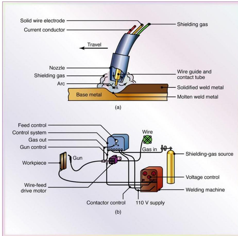
(a) Schematic illustration of the gas metal-arc welding process, formerly known as MIG (for metal inert gas) welding. (b) Basic equipment used in gas metal-arc welding operations.
