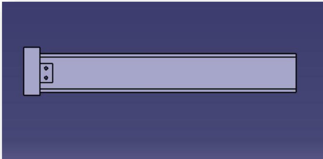
Figure 3 Front view of the I-beam
