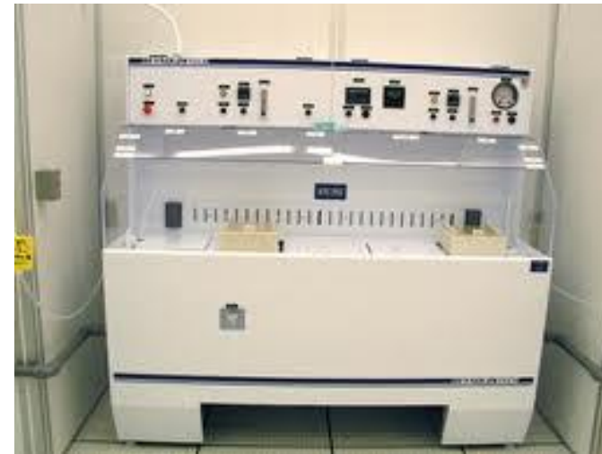
A 5-compartment wet etching table
