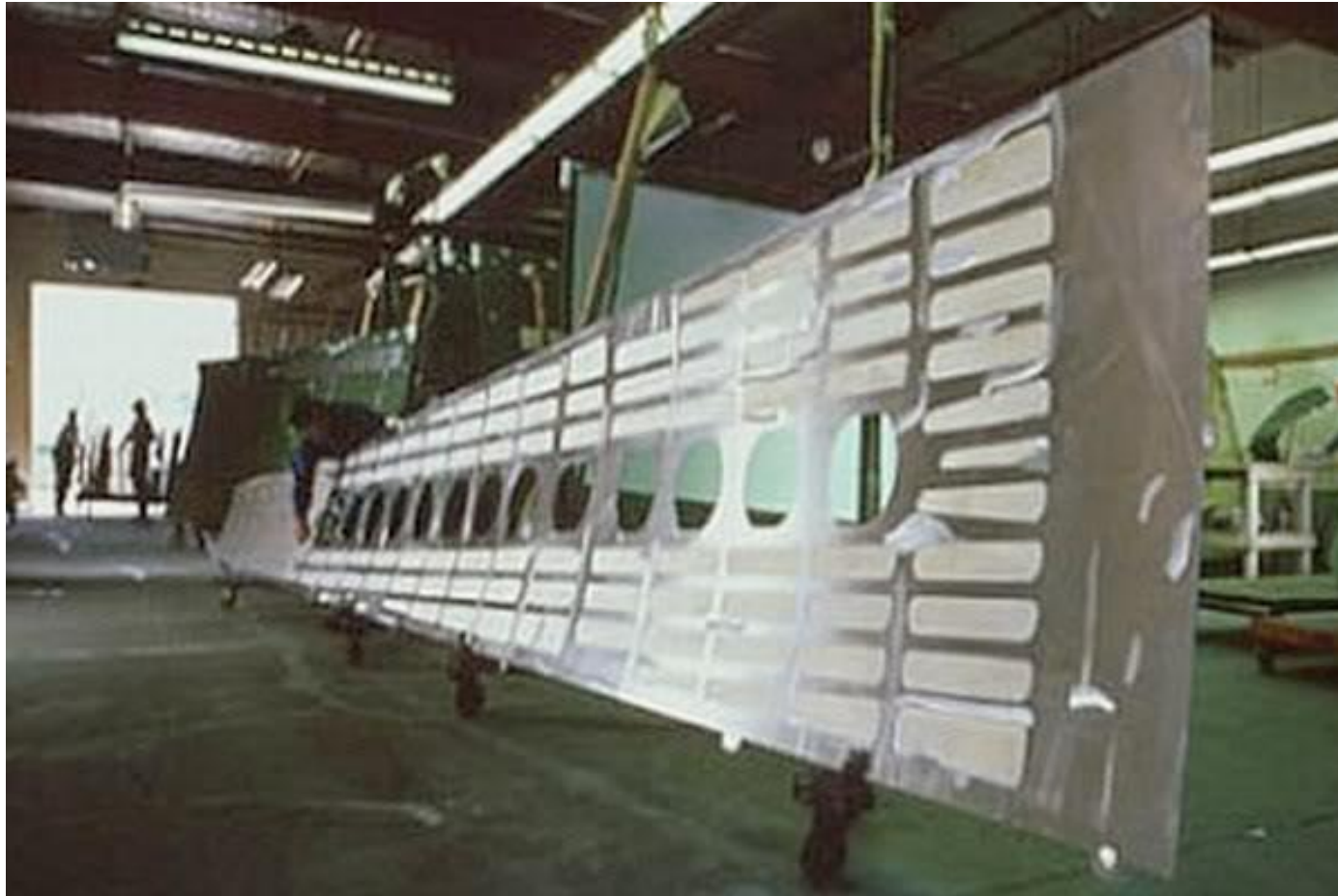
Figure: Chemically milled fuselage skin panel
