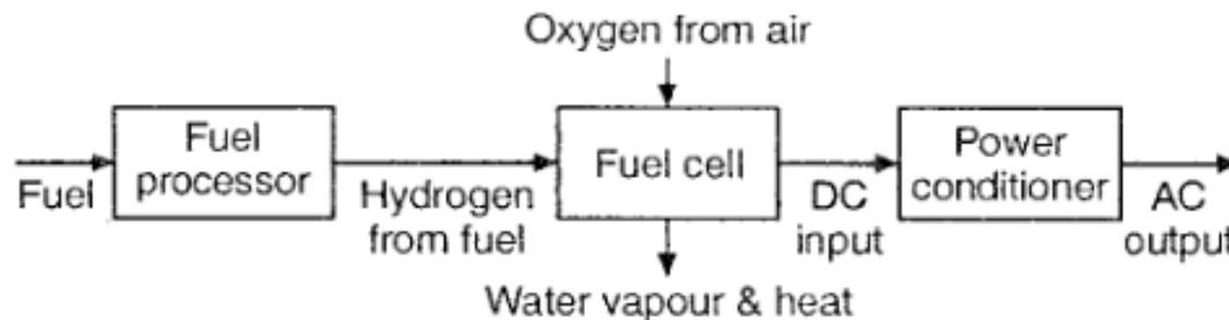
Energy flow diagram in a fuel cell.
