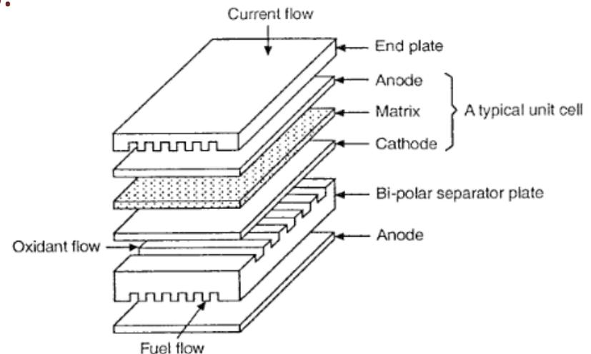
Schematic of repeating elements in a PAFC stack.
