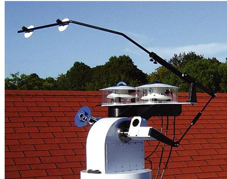
Diffuse solar irradiance measured by adding a shadowing device to a pyranometers, which blocks the direct component of total irradiance.
