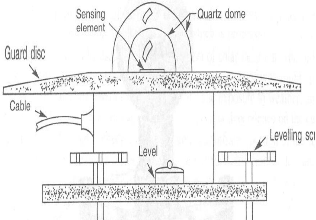
Crossed-section of Pyranometers
