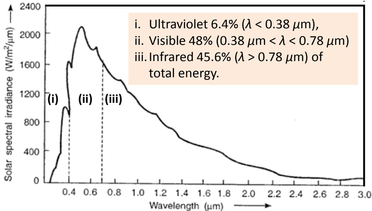
**Extraterrestrial radiation:** solar radiation in the absence of atmosphere
