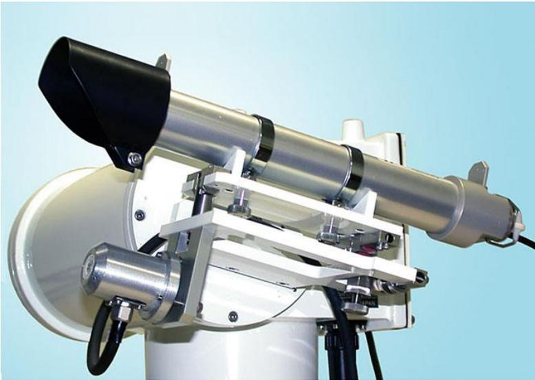
Pyrheliometer measures direct component of solar irradiance, which is important when installing concentrating collectors.
