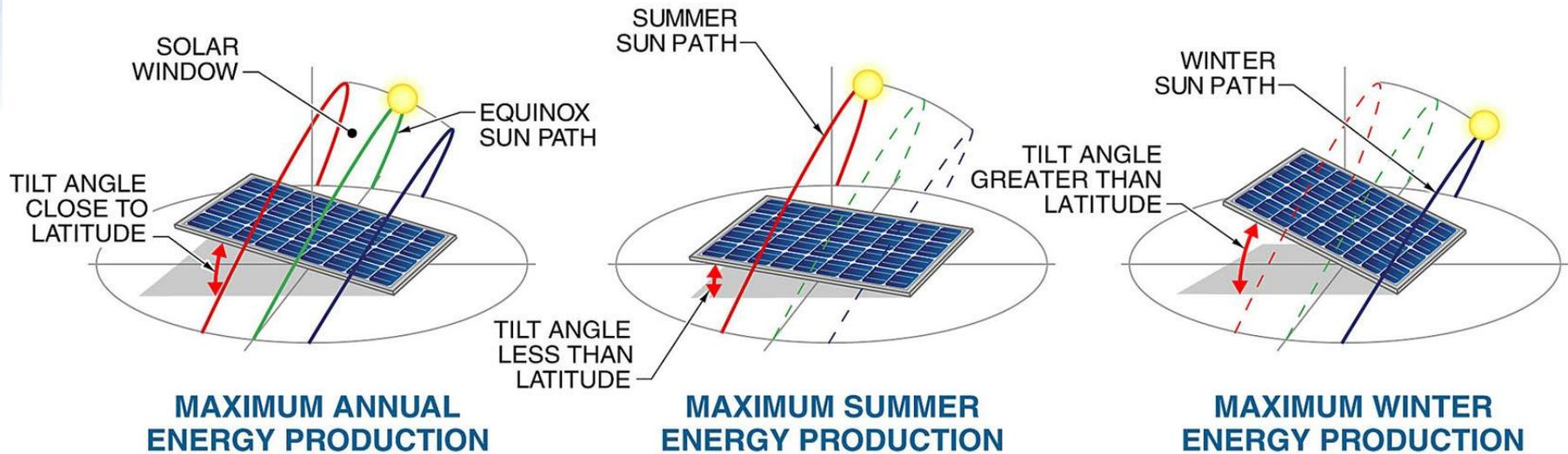
Energy production at certain times of the year can be optimized by adjusting the array tilt angle.
