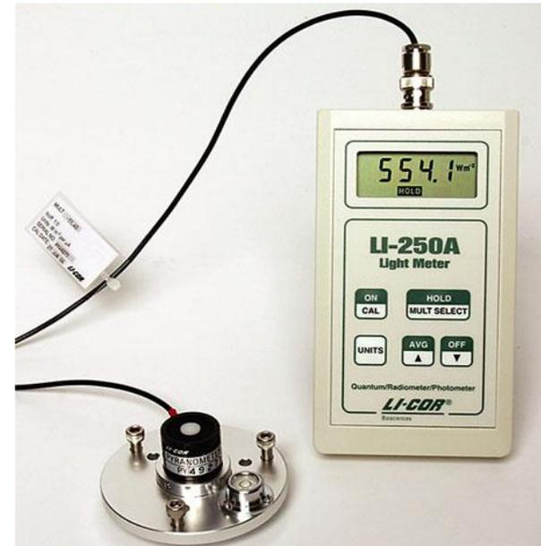
Handheld pyranometers use less precise sensors, suitable for field measurements.
