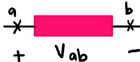
The voltage across an element is the work (energy  $W$ ) required to move a unit positive charge from the  $-ve$  terminal to the  $+ve$  terminal.
