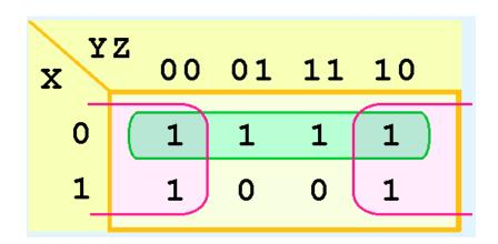
• Simplified function is:  $F(X,Y,Z) = \overline{X} + \overline{Z}$
