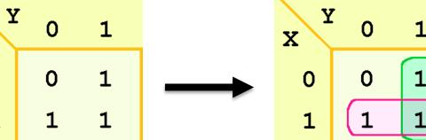
$$F(x,y) = x + y = \overline{x}y + x\overline{y} + xy$$
