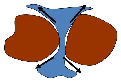
Sub-base must be free-draining so that water is readily removed. If too much of fines, the base becomes saturated (with water ), high stressed may be created by water that fills in the pores space. Resulting to a less frictional strength between particles (aggregate ).
