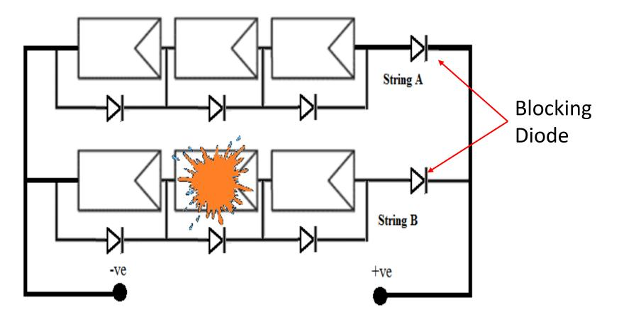
Placement of blocking diode
