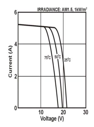
The V<sub>mp</sub> decreases by approximately 0.5% per °C as the PV cell temperature increases above 25°C
