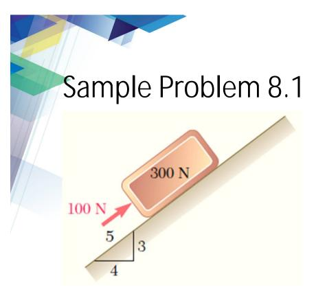
A 100-N force acts as shown on a 300-N block placed on an inclined plane. The coefficients of friction between the block and plane are  $\mu_s = 0.25$  and  $\mu_k = 0.20$ . Determine whether the block is in equilibrium and find the value of the friction force.
