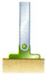
Frictionless pin or hinge
