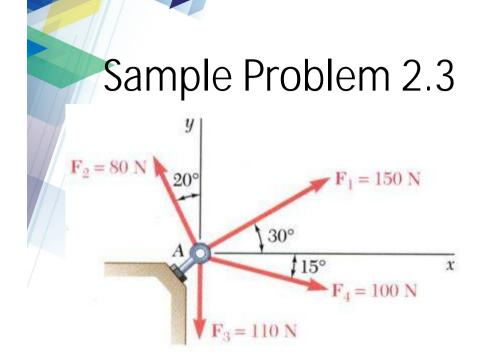
Four forces act on bolt *A* as shown. Determine the resultant of the force on the bolt.
