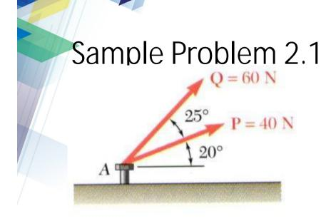
The two forces act on a bolt at A. Determine their resultant by using
