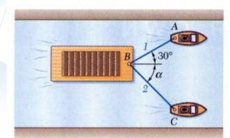
A barge is pulled by two tugboats. If the resultant of the forces exerted by the tugboats is 5000 lbf directed along the axis of the barge, determine:
