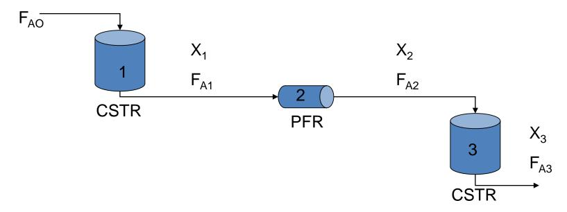
$$X_n = \frac{Moles\ of\ A\ reacted\ up\ to\ reactor\ n}{Moles\ of\ A\ feed\ to\ first\ reactor}$$
