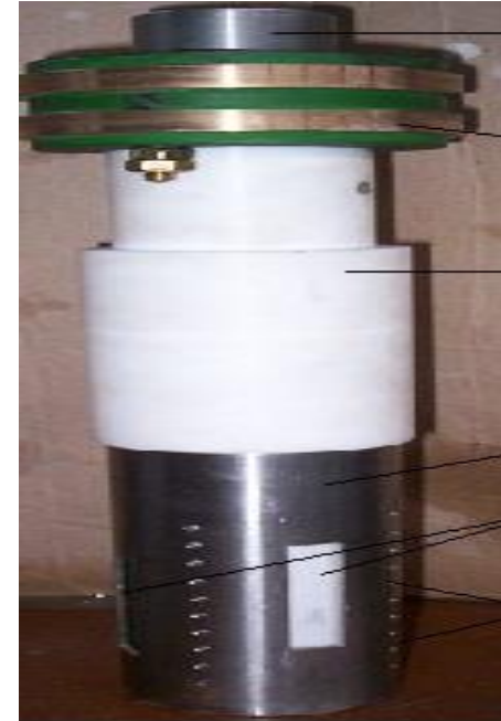
Fig. (a) Schematic and (b) photograph of a typical tool for finishing internal cylinders by ECH
