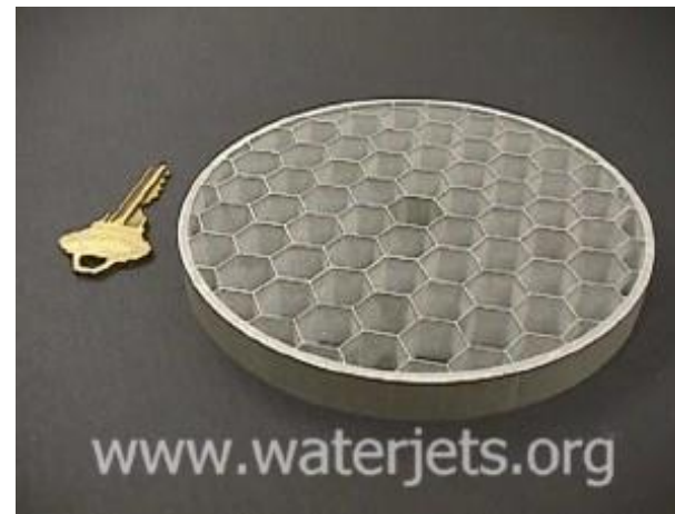
Honeycomb part; Aluminium, t = 13 mm, wall thickness = 0.6 mm
