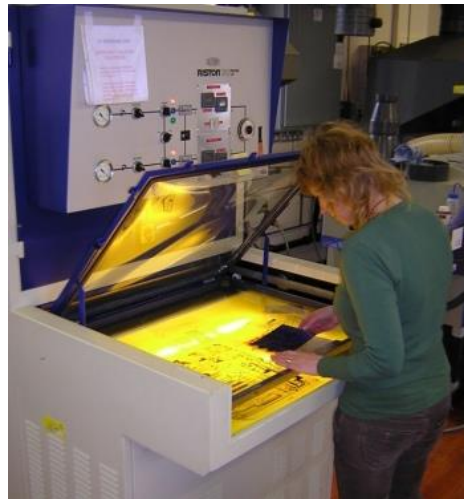
Figure: UV exposure unit
