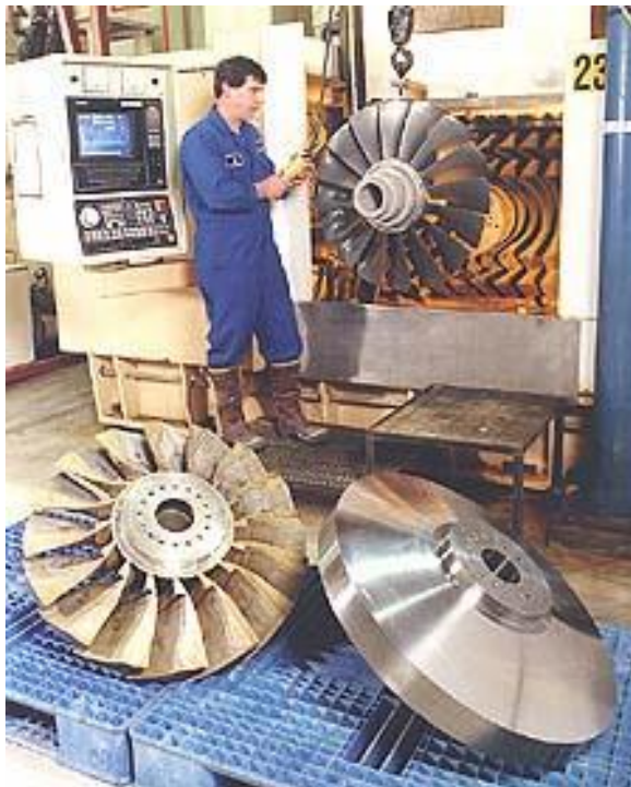
Figure: ECM of turbine blisk in 3 stages - forging (lower right), rough cut (lower left), and finish cut by ECM [Sermatech Cincinnati, USA]
