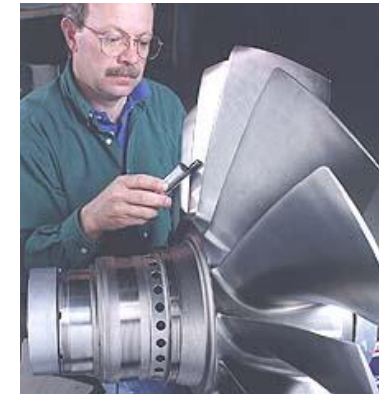
Figure: Compressor blisk by ECM in F110 fighter engine feature both reduced mass and complexity compared to individually bladed rotors
