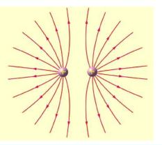
Electric field line for two positive charges, or two negative charge. Notice that the electric field is zero in the midpoint between the two charges
