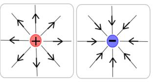
Electric field lines pointing away from positive charge, and pointing into negative charge. A higher charge can be represented by drawing more lines around the charge.
