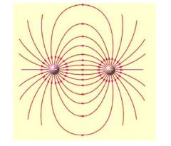
Electric field line for a positive charge and a negative charge placed nearby. This is also called a dipole.
