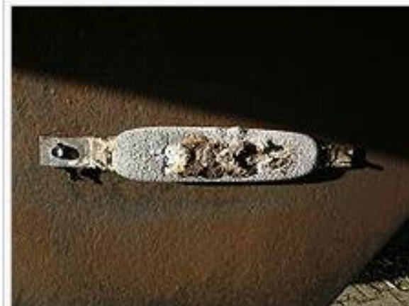
Galvanic sacrificial anode attached to the hull of a ship, showing corrosion.
