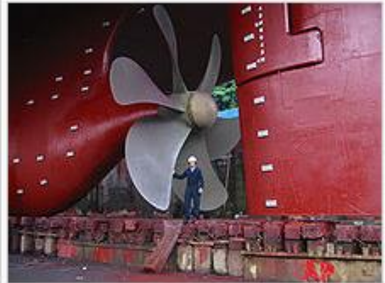
The white patches visible on the ship's hull are zinc block sacrificial anodes.
