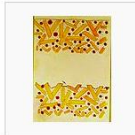
Figure 1.2: Diagram showing paint pigments in a resin matrix. It can be seen that weathering only removes the smaller pigments, resulting in the colour change
