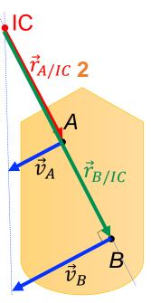
Velocity directions are parallel to each other in the same direction Velocity directions are parallel to each other in the opposite direction
