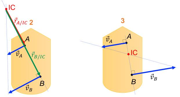
Velocity directions are parallel to each other in the same direction Velocity directions are parallel to each other in the opposite direction
