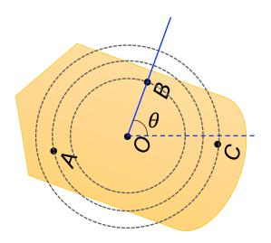
Linear motionAngular motion $v = \frac{ds}{dt}$  $\omega = \frac{d\theta}{dt}$  $a = \frac{dv}{dt}$  $\alpha = \frac{d\omega}{dt}$ ads = vdv $\alpha d\theta = \omega d\omega$
