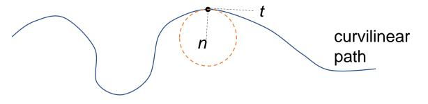
*t* : tangential axis – tangent to the path *n* : normal axis – point towards the centre of the arc
