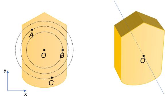
The path of motion of any point (particle) on the rigid body is **ALWAYS CIRCULAR**
