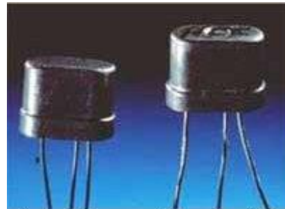
The first commercially produced silicon transistor, developed by Texas Instruments in the early 1950s. Courtesy: Texas Instruments.
