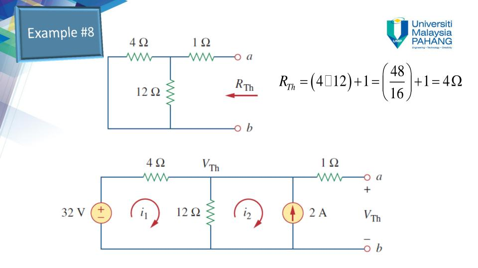
To find  $V_{Th}$  apply mesh analysis to the two loops
