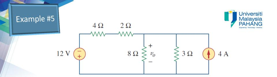
Combining the 4  $\Omega$  and 2  $\Omega$  in series and transforming 12 V voltage source
