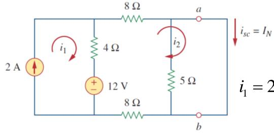
we ignored the 5  $\Omega$ resistor because it has been short circuit
