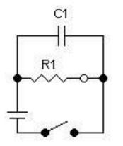
There is a capacitor in parallel with the resistor and light bulb. The way the capacitor functions is by acting as a very low resistance **load** when the circuit is initially turned on. This is illustrated below:
