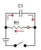
vi. As time goes on, the capacitor's charge begins to drop, and so does its voltage. This means less current flowing through the resistor:
