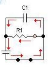
iii. As a capacitor charges, its resistance increases as it gains more and more charge. As the resistance of the capacitor climbs, electricity begins to flow not only to the capacitor, but through the resistor as well:
