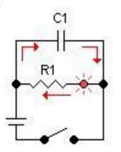
v. Once the voltage source is disconnected, however, the capacitor acts as a voltage source itself:
