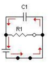
Initially, the capacitor has a very low resistance, almost 0. Since electricity takes the path of least resistance, almost all the electricity flows through the capacitor, not the resistor, as the resistor has considerably higher resistance.
