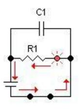
iv. Once the capacitor's voltage equals that of the battery, meaning it is fully charged, it will not allow any current to pass through it. As a capacitor charges its resistance increases and becomes effectively infinite (open connection) and all the electricity flows through the resistor.
