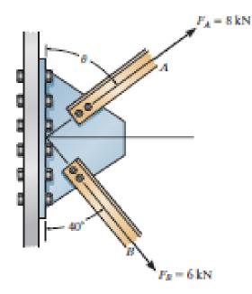
T5) Determine the angle of  $\theta$  which connecting member A to the plate so that the resultant force of  $F_A$  and  $F_B$  is directed horizontally to the right. Also, determine the magnitude of the resultant force
