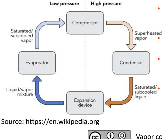
System that transfer the heat from a low-temperature reservoir to a high-temperature one.
