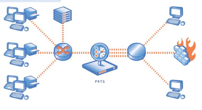
The Simple Network Management Protocol (SNMP) is the basic method of gathering bandwidth and network usage data. It can be used to monitor bandwidth usage of routers and switches port-by-port as well as device readings like memory, CPU load etc.
