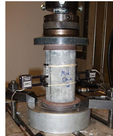
Simple compressive stress
