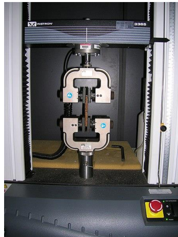
Simple tension stress
