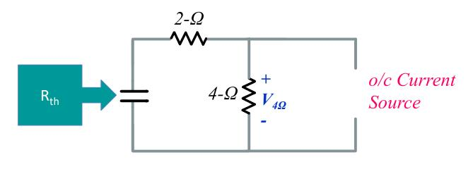
$$R_{th} = R_{2\Omega,4\Omega} = 6-\Omega$$
