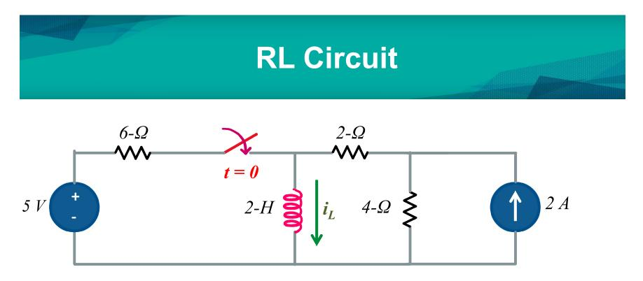
The switch in the circuit has been opened for a long time before it close at t=0. Find  $i_{L}(t)$  for t  $\geq$  0.
