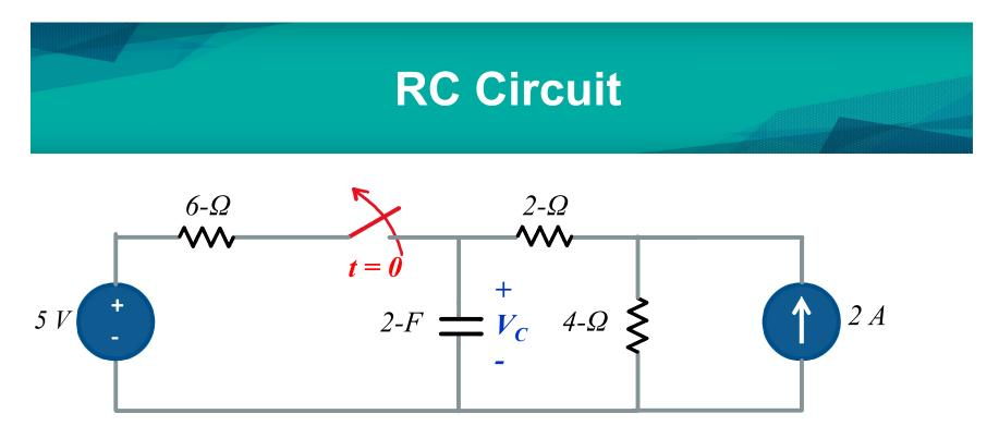
The switch in the circuit has been closed for a long time before it open at t=0. Find  $V_c(t)$  for t  $\ge 0$ .
