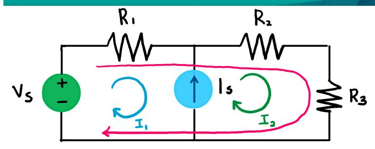
KVL at Supernode:  $-V_s + I_1R_1 + I_2R_2 + I_2R_3 = 0$
