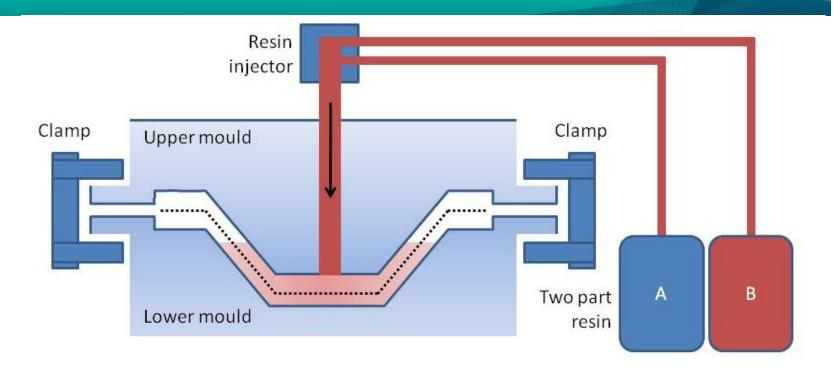
Dry woven roving is laid into the lower mould and the upper mould is fixed in place. Low viscosity resin + catalyst is injected under pressure into the mould cavity, where it permeates the fibres. The composite cures whilst in the mould. This technique is used for low volume production in the manufacture of components such as boat hulls, car parts, etc.
