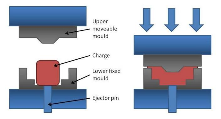
Compression moulding can be used to shape polymer matrix composites. The charge is placed between two steel platens and is heated and cured under pressure. This technique produces components with a high quality surface finish and also has a short cycle time, making it ideal for processes where a high throughput is required. For lower volume production, high machine costs may make this process prohibitively expensive.
