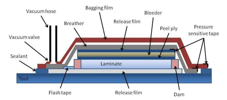
The vacuum bagging technique can be used to improve the quality of composites produced by the wet lay-up method. A bagging film is placed around the laid-up composite material and is secured to the tool surface with sealant. Air is evacuated from the bag, leaving the composite under an external pressure of up to 1 atmosphere. This forces resin into any remaining voids and helps to ensure an even distribution. Higher viscosity resins can be used in comparison to the wet lay-up technique.
