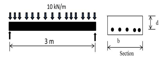
A 3 m span simply supported slab with effective depth d = 125 mm carries an ultimate action of 10 kN/m per m width. The provided tension reinforcement steel is H8-150 bar. Use  $f_{ck} = 25$  N/mm<sup>2</sup> and  $f_{yk} = 500$  N/mm<sup>2</sup>. Verify shear reinforcement for this section.
