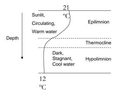
Thermal stratification: Region of sharp thermal gradient
