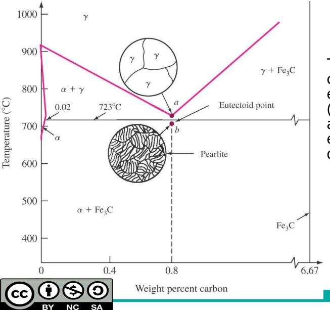
The microstructures of carbon steel at eutectoid composition (0.77% carbon), above and below the eutectoid temperature of 727 °C.
