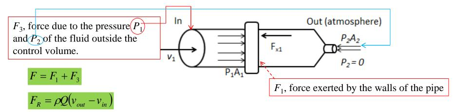
The force exerted by the fluid on the solid body will be equal and opposite to F<sub>1</sub>, so that the R = -F<sub>1</sub>
