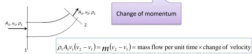
• If  $\rho_2 = \rho_1$  and according to continuity principle and the Newton Second Law; the rate of change between section 1 and 2 is :
