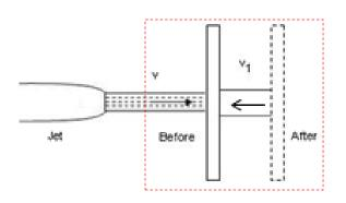
Effective velocity,  $v_e$  $v_e = v + v_1$
