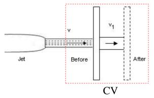
Efective velocity,  $v_e$   $v_e = v - v_1$ Efective discharge,  $Q_e$   $Q_e = Av_e$  $Q_e = A(v - v_1)$
