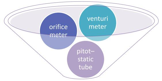
Make use of the pressure difference between two points in the flow to give an indication of the flow rate.
