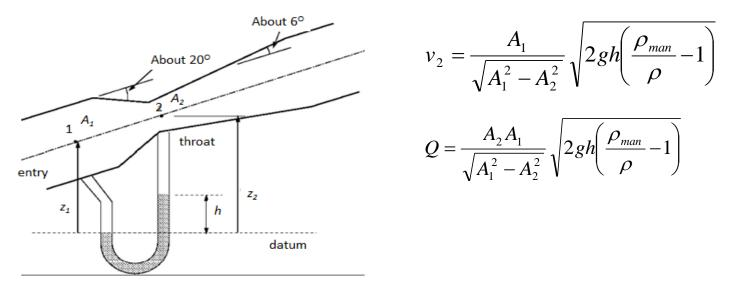
The discharge formula given above is the theoretical discharge. Thus in order to get the actual discharge, the discharge coefficient C<sub>d</sub> must be known.
