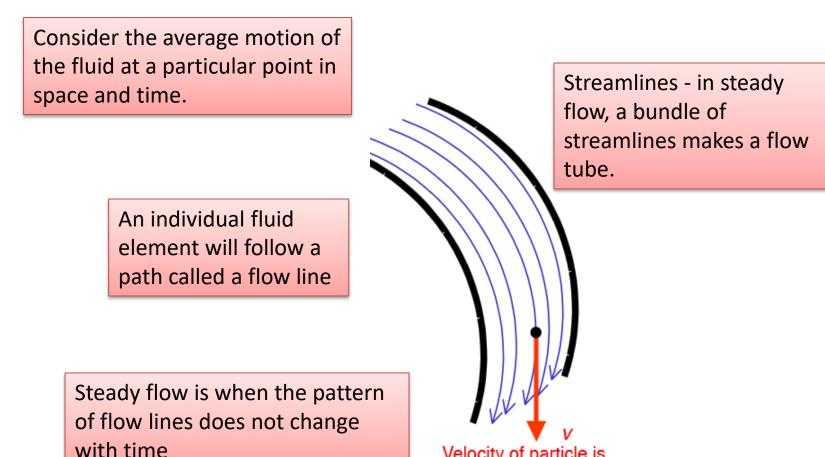
Velocity of particle is tangent to streamline
