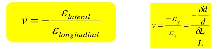
Poisson' ratio is dimensionless and most metal has a value of v between 1/3 and 1/4, the largest possible value of v is 1/2
