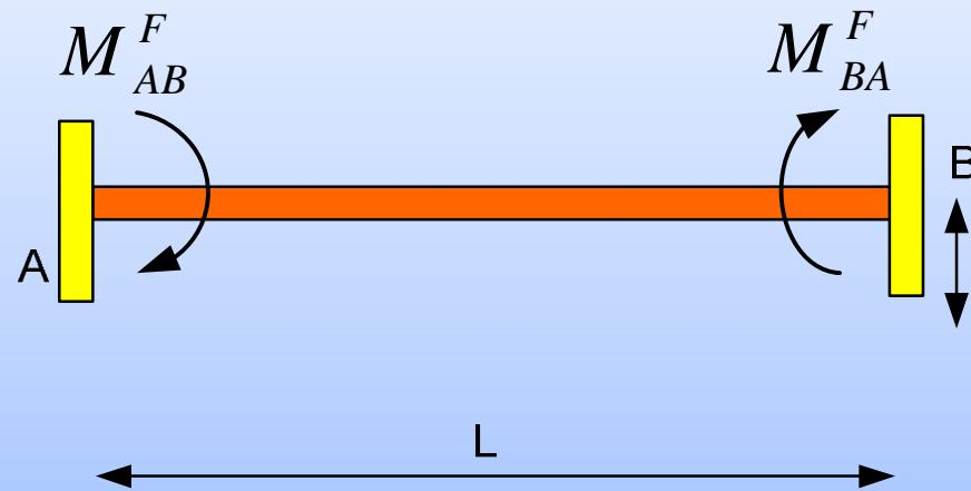
Moment cause by external load whilst the both support are fixed.
