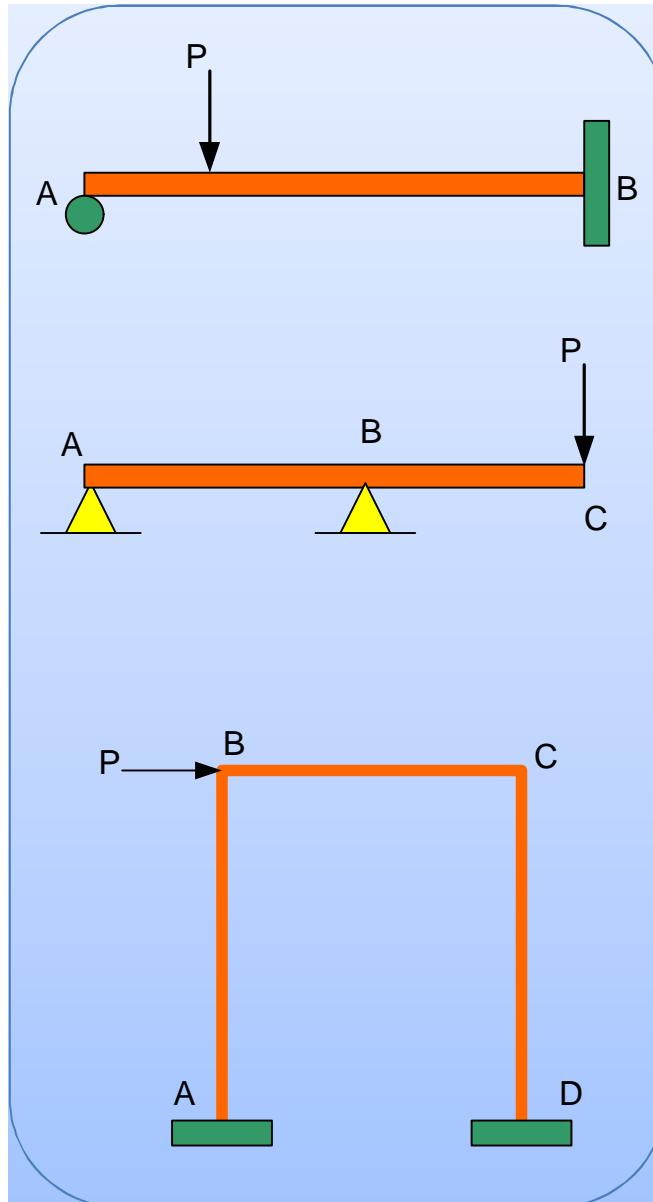
*When load  $P$  is applied to the beam, will cause node A to rotate, while node B is completely restricted from moving.*
