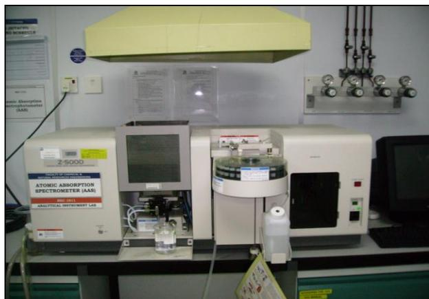
Figure 1 Polarized Zeeman Atomic Absorption Spectrophotometer (Model Z-5000 Series)
