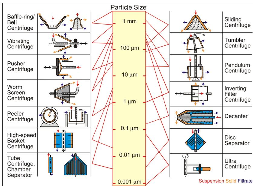
Fig. 6. Centrifuge selection alternatives and possible correlation to particle size. Graphic provided by Karsten Keller of DuPont.
