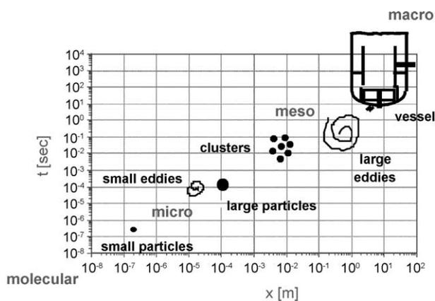
Fig. 5. Range of time and size scales encountered in crystallization processes. Graphic provided by Daniel Green of DuPont.
