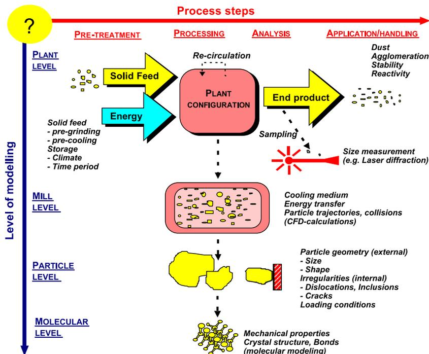
Fig. 7. Application of modeling to a grinding circuit. Graphic provided by Erik Gommeren of DuPont.
