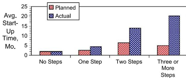
Fig. 4. Start-up time versus new process steps (from Merrow [3]). New process steps are defined as having never before been used commercially.
