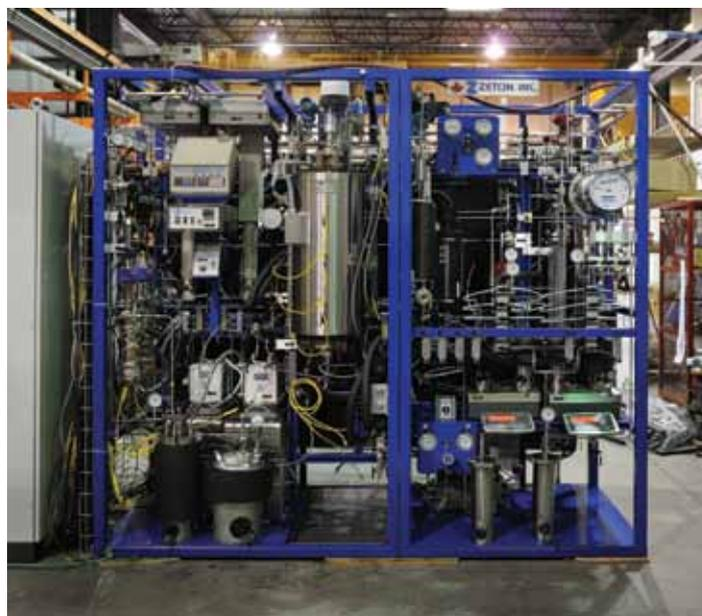
A novel lab scale ebullated bed reactor system for continuous bio-oil upgrading
